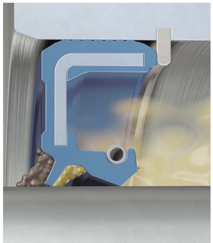
A well-established team: Combined, the seal and the lubricant help to reduce the hazards of leakage
