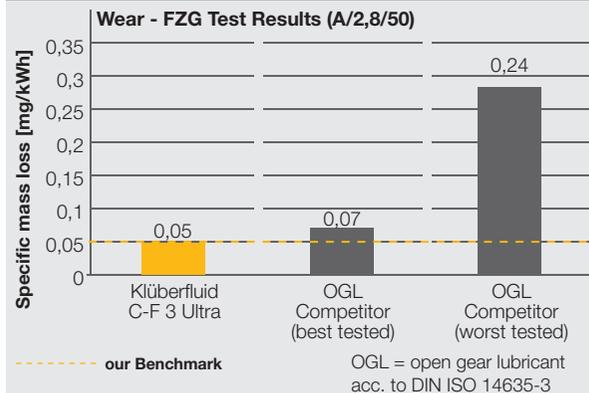
In the optional FZG wear test, Klüberfluid C-F 3 Ultra shows 30 % less wear than the best competitor product and 60 % less than the average of all tested competitor products.
