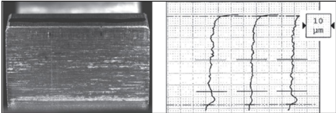
**Fig. 3: Pinion type C-GF with measurement of the profile, nearly no micropitting failure.**
