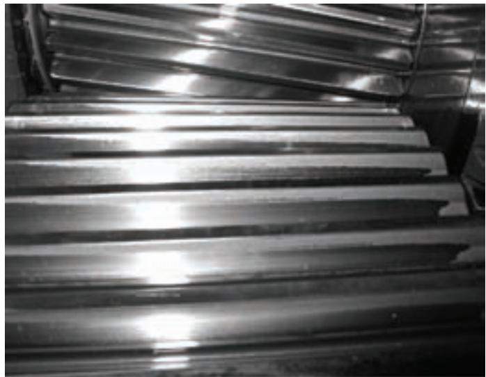
Fig. 2: Micropitting gear failure of an industrial gearbox.
