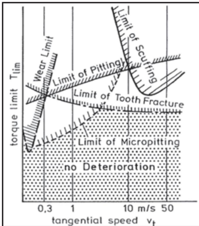
Fig. 1: Typical limits of the load-carrying capacity for case hardened gears.
