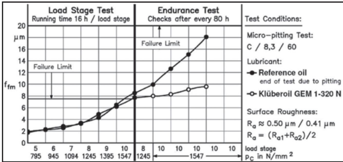
Fig. 7: Stopping micropitting by using a high-performance gear oil (mineral oil).
