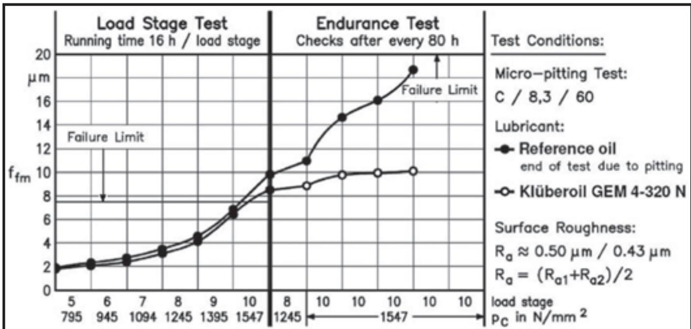
Fig. 8: Stopping micropitting by using a high-performance gear oil (polyalphaolefin).
