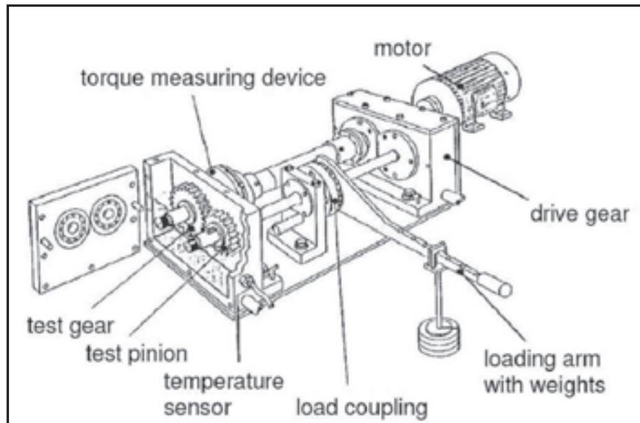
**Fig. 6: FZG back-to-back gear test rig.**
