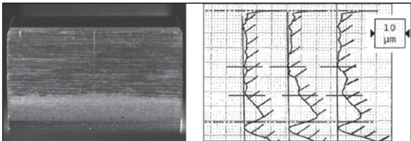
**Fig. 4: Pinion type C-GF with measurement of the profile, micropitting failure in the range of the failure criterion.**
