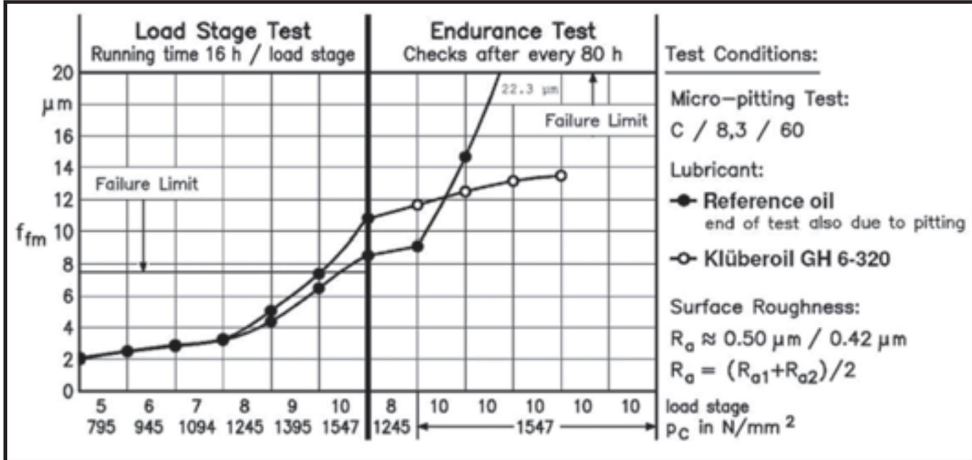
Fig. 9: Stopping micropitting by using a high-performance gear oil (polyglycol).
