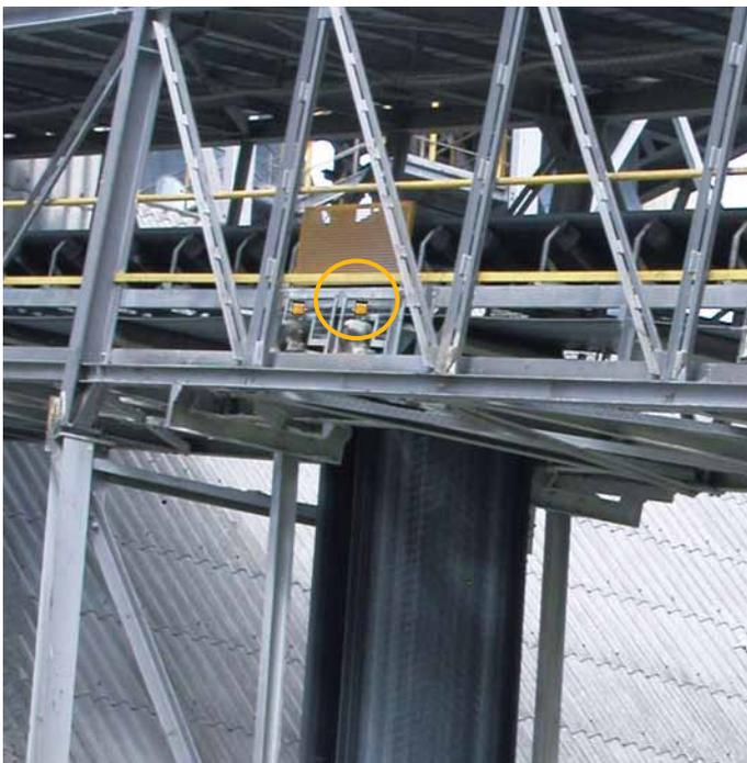
(above left) **Belt conveyor / gravity take-up pulley**
