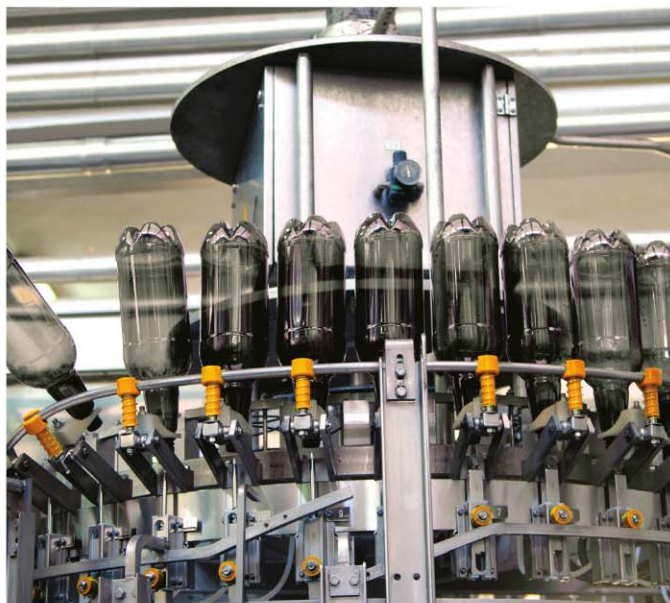
Bottle filling machine in operation: A critical area where food machinery lubricants have to be used.
