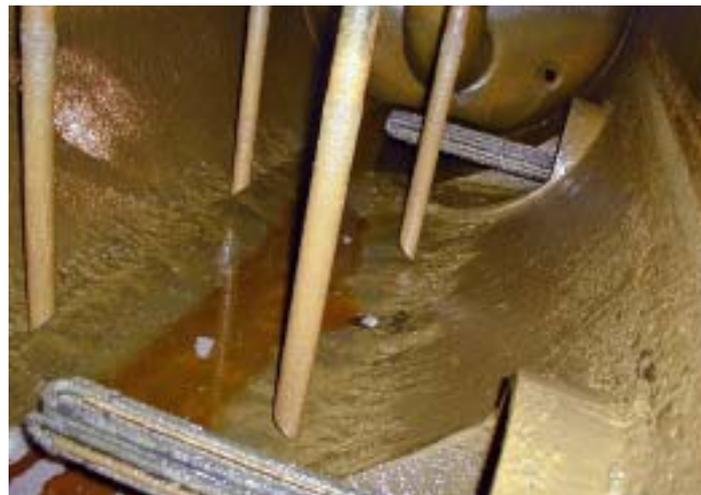
*Oil container of a process gas compressor, covered with greenish sludge from reactions between the lubricating oil and the process gas*
