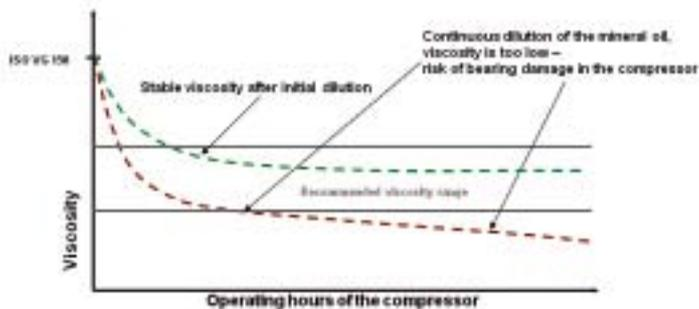
*Schematic viscosity curve of a polyglycol oil compared to a mineral oil when a hydrocarbon/gas mixture is compressed*
