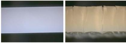
② Polyoxymethylene homopolymer after storage under dry conditions (left) and after exposure to lubricant (right), 1000 h/100 °C
