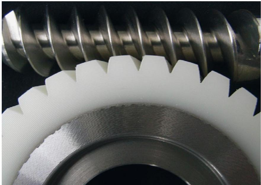
④ Electromechanical power steering system with a worm made of steel and a worm wheel made of polyamide 6.6
