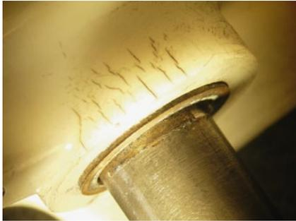
③ Typical tension crack damage
