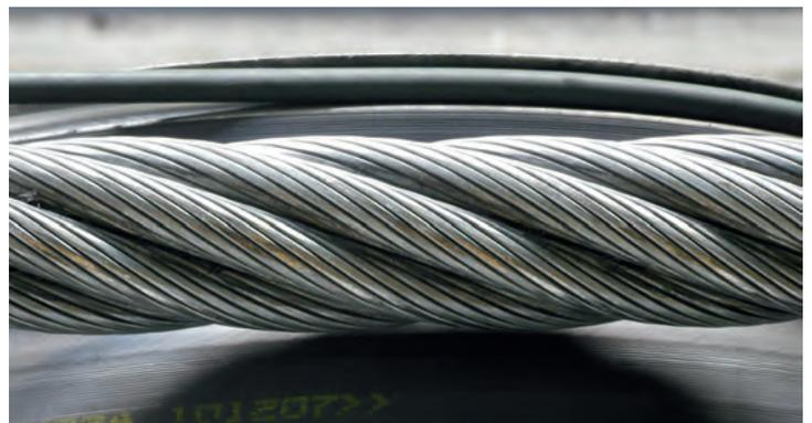
Wire rope on roller with elastomer lining
