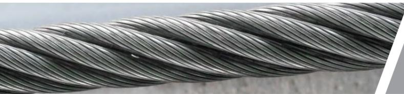
**In Europe, a wire rope for people transportation applications should be manufactured according to EN 12385-8. This norm contains indications for the lubricant to be used as the first fill:**
