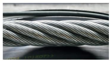
Wire rope on roller with elastomer lining
