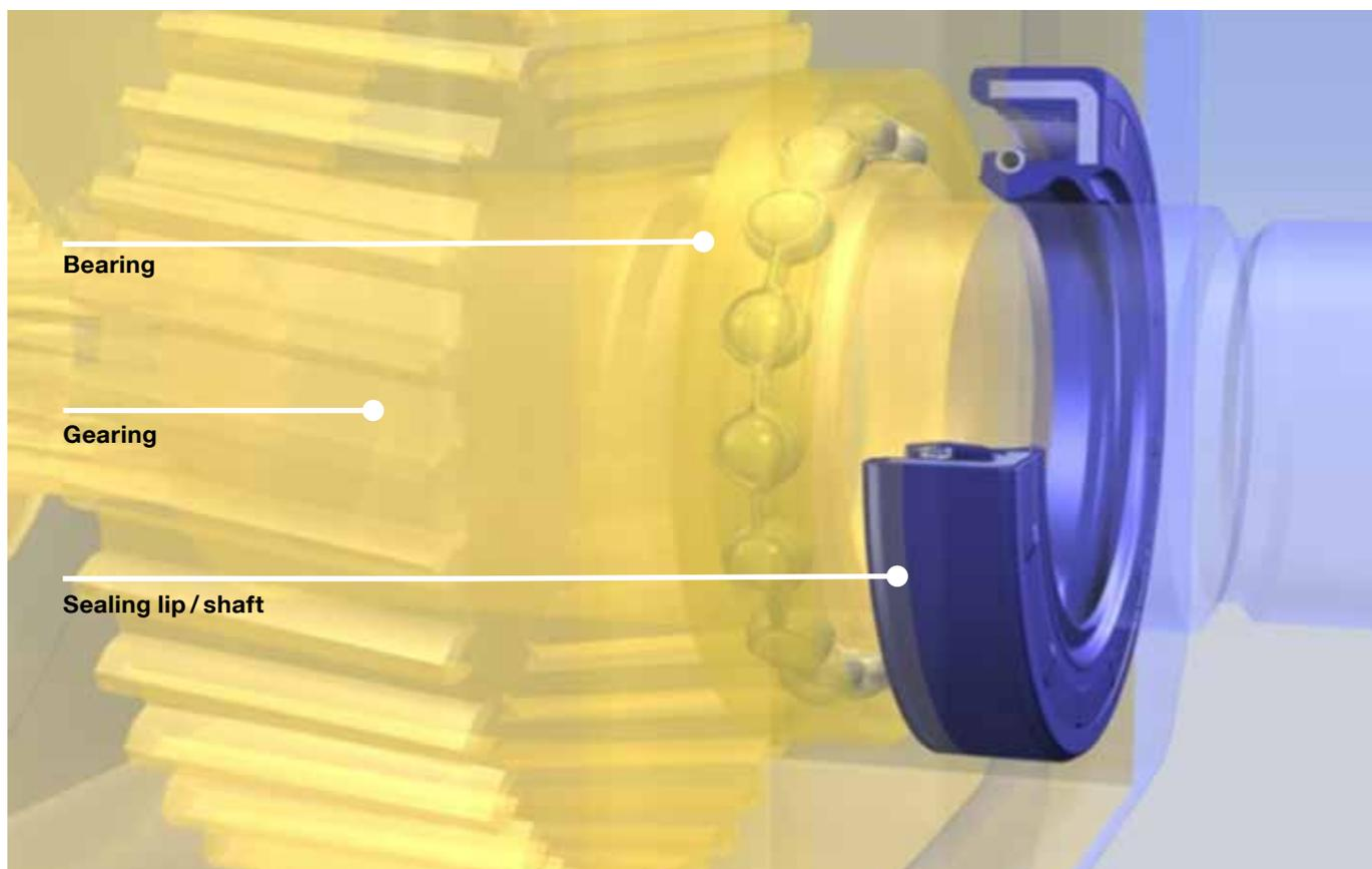
With Lube & Seal, the sealing lip tribosystem is now integrated into the lubricant development process.
