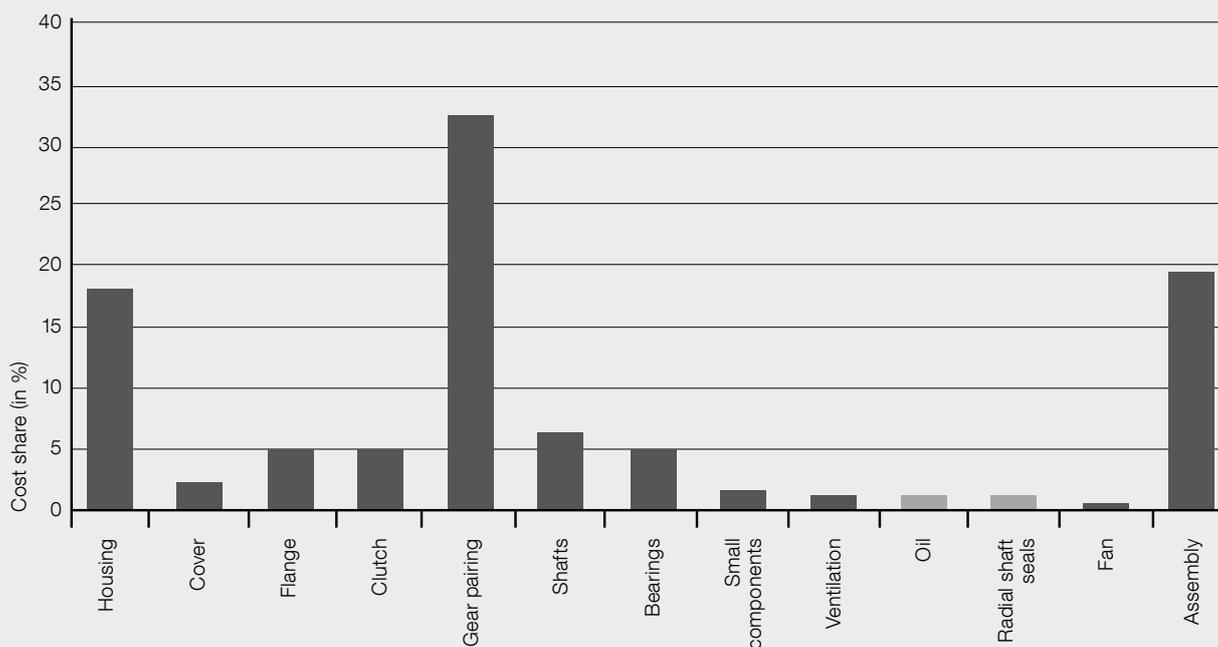
Cost distribution in the manufacture of gearboxes (example: worm gearbox)
