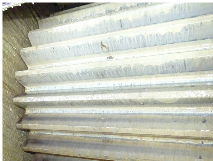
Open gear lubricated with Klübersynth OA 98-15000
