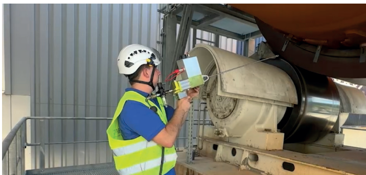
Lubricating the ring gap using ss. LUBAC Ring Star
