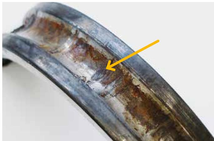
Wear marks caused by vibrations in stationary bearings – so-called False Brinelling
