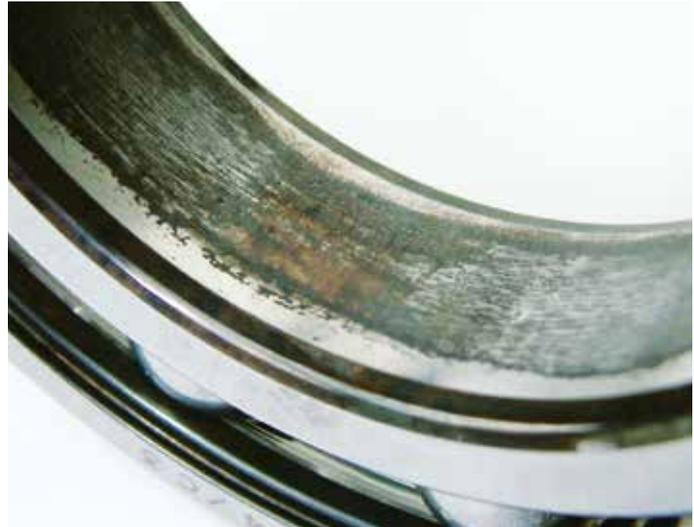
Fretting corrosion on inner ring
