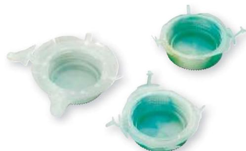
By using a suitable purging compound neither flushing (picture on the top) nor short shots (picture below) will occur.
