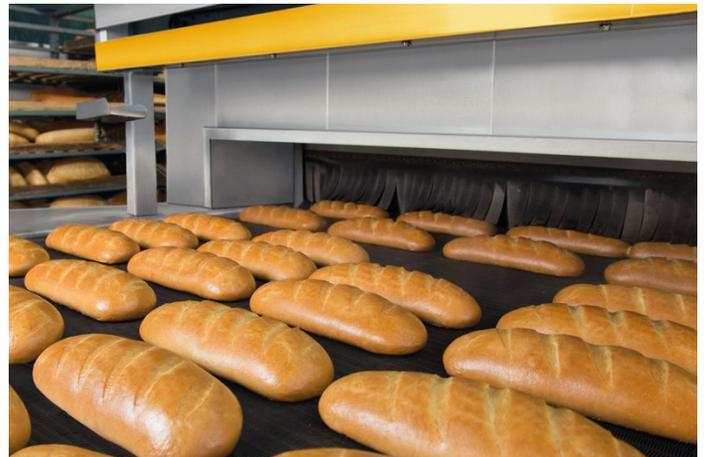
Conveyor chains in bakery ovens are exposed to extreme temperatures upward of 1000°F (537°C), which can significantly challenge typical food-grade lubricants, such as synthetic esters that can evaporate at temperatures above 500-600°F (260-315°C).
